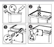
Ensure all stand/feet screws are tightened securely.
